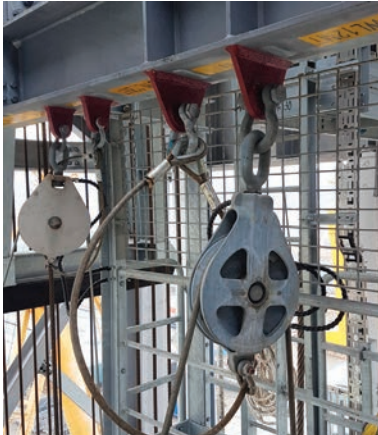
Figure 12: Block with safety securing device
