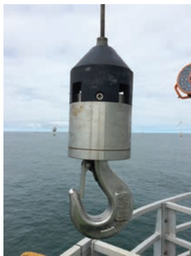
Figure 16: Hooks for lifting should always be equipped with a safety device to prevent the load becoming detached from the hook
