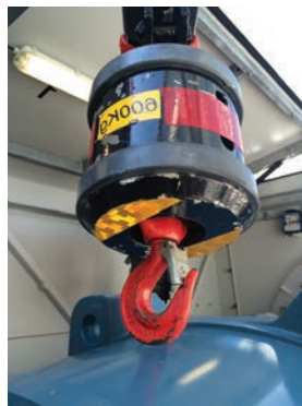
Figure 16: Hooks for lifting should always be equipped with a safety device to prevent the load becoming detached from the hook
