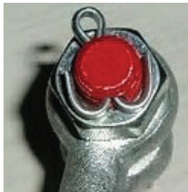
Figure 11: Ensure pins are properly splayed to reduce the risk of snagging and injury
