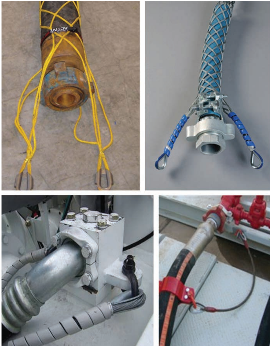
Figure 17: Hanging hoses and service loops present a safety problem (sourced from DROPS)
