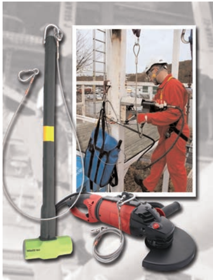
Figure 4: A variety of tools and hand-held machinery is available specifically for heavy duty use at height (sourced from DROPS)
