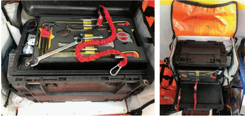
Figure 5: Tool cabinets for work at height are now readily available and employed on many facilities
