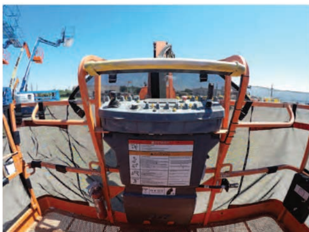
Figure 8: Ensure the MEWPs do not get congested and consider installing a suitable method of enclosing the unit when working at height
