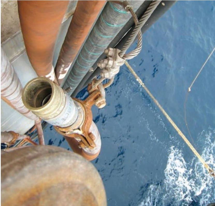
Figure 9: Home-made lifting device with a poor clamp selection (sourced from DROPS)
