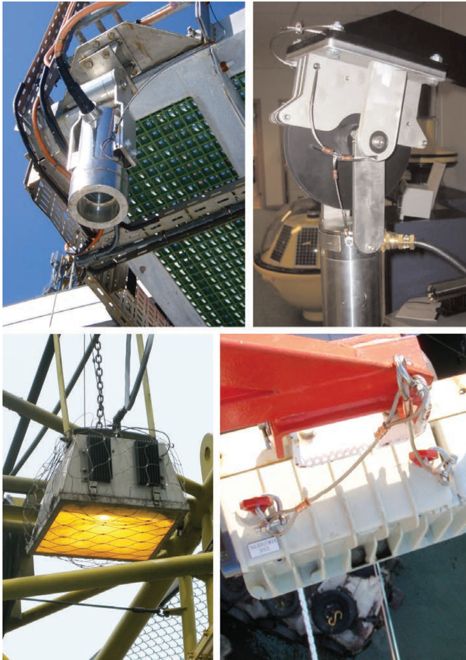
Figure 33: Crane boom camera and pivoting floodlamps (sourced from DROPS)
