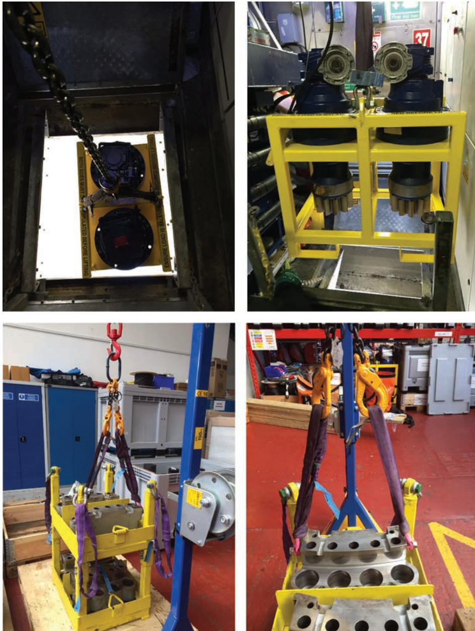
Figure 19: Specialist lifting frames (yaw gear motors and yaw callipers)
