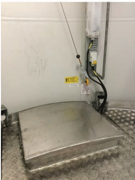
Figure 23: Ensure all hatches, doors and access panels are correctly seated and secured
