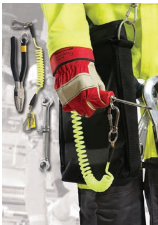
Figure 3: Lanyard attachment points (moveable, spring clip or fixed) should be selected according to size and weight of tool (sourced from DROPS)
