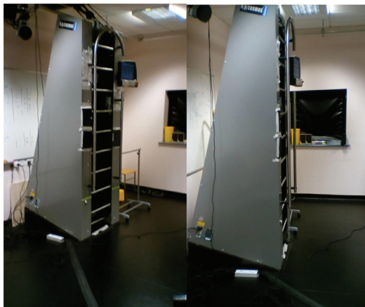
Figure 3.3.2.1: Ladder ergometer. HP Cosmos ladder with wedge underneath to create a vertical ladder treadmill
