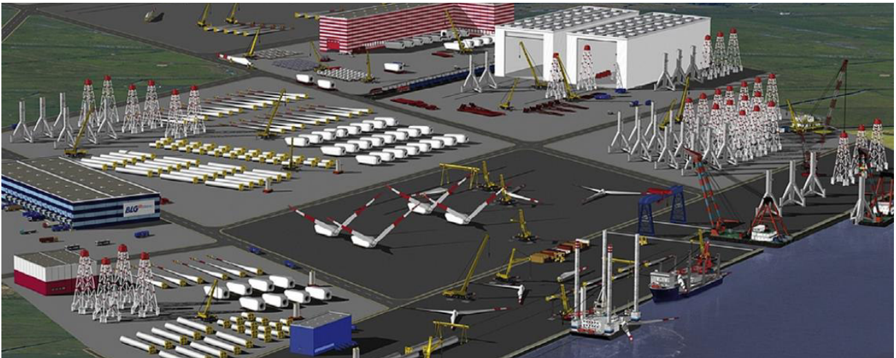
Figure 3-47 Example of onshore pre-assembly site (harbour) for offshore wind farm installation (Asgarpour, 2016).
