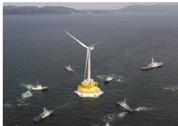
Figure 2-12 Tow out of Fukushima Hamakaze 5MW Hitachi wind turbine (Trabish, 2016)
