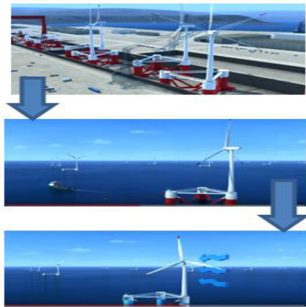
Figure 3-78 Tri-floater vertical transportation concept (Principle Power, 2011)
