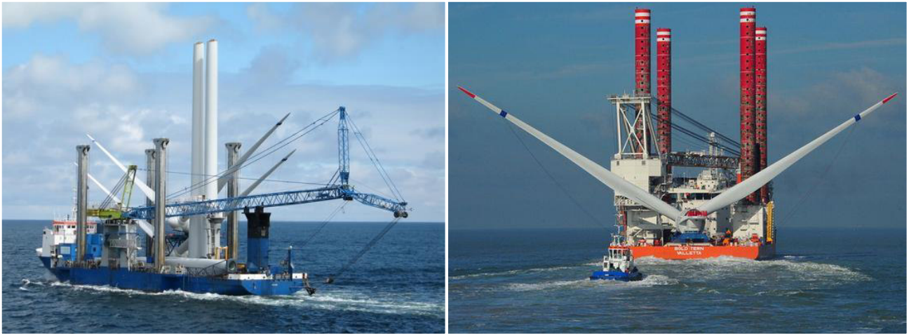
Figure 3-49 BE configuration offshore transportation examples (Fred. Olsen Windcarrier, 2013; Uraz, 2011)
