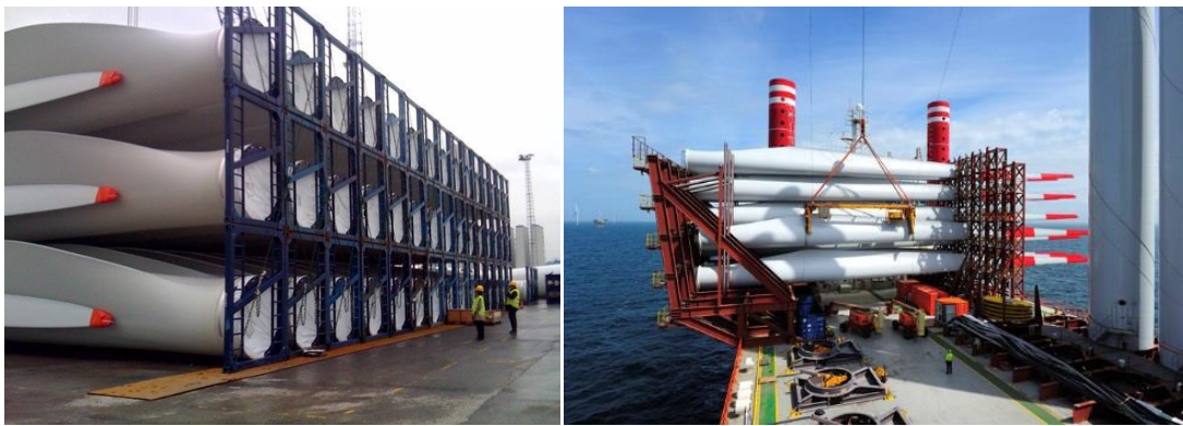
Figure 3-63: Blade “cage”, transportation gathering structure examples (Fred. Olsen Windcarrier, 2017; Lawson, 2012)
