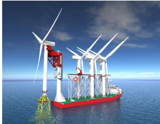
Figure 2-10 Installation vessel for fully-assembled wind turbines (Vuyk Engineering Rotterdam b.v., 2017)
