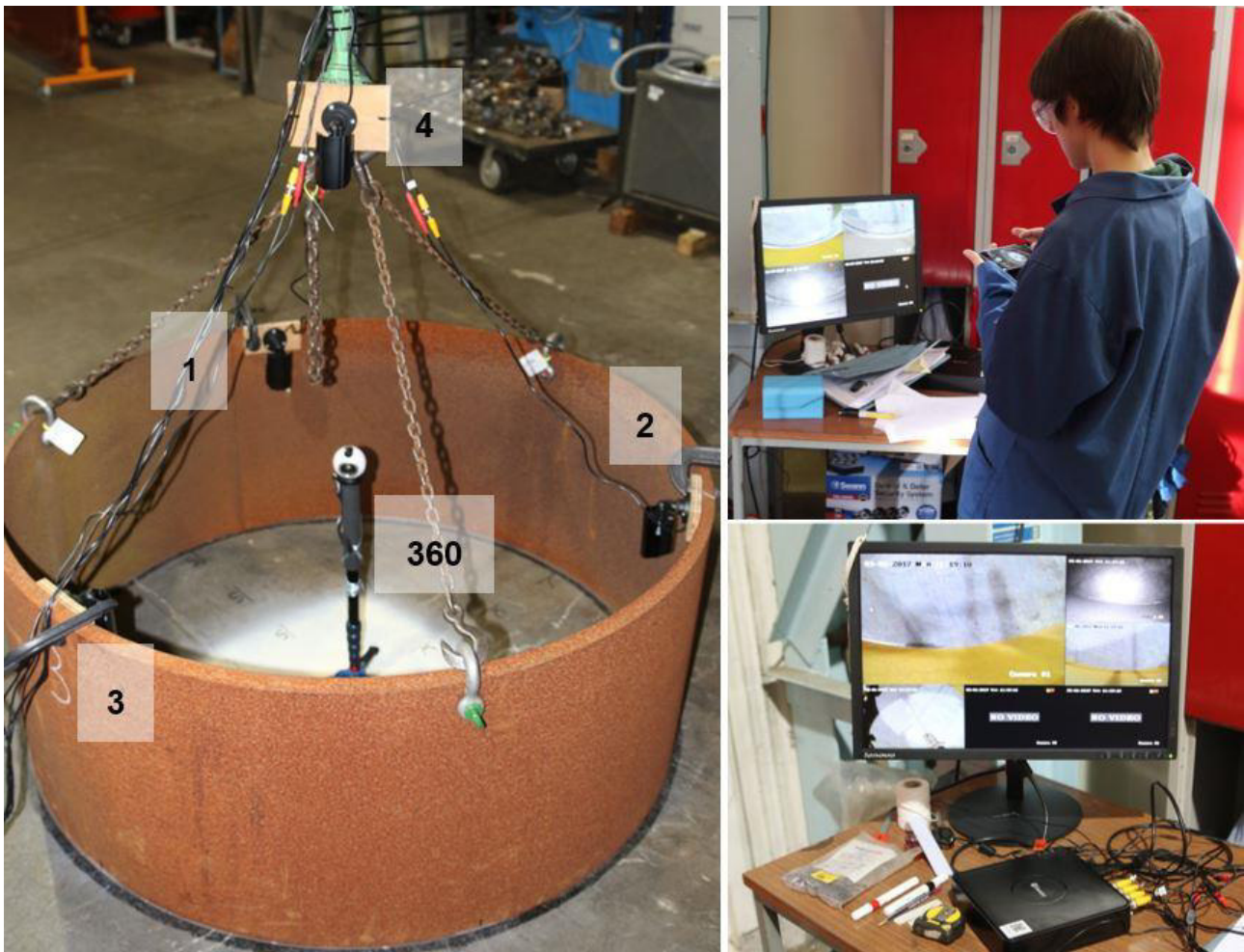
Figure 3-18 Left) Set-up of the cameras and crane system. Top right) typical view of 360 camera feed and monitor. Bottom right) Monitor feed of cameras 1, 2, 3 & 4.
