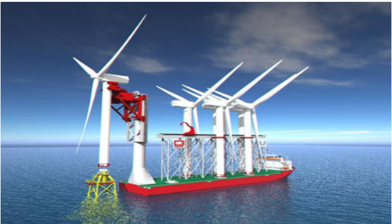
Figure 3-77 Fully pre-assembly using special vessel (single lift) (Vuyk Engineering Rotterdam b.v., 2017)
