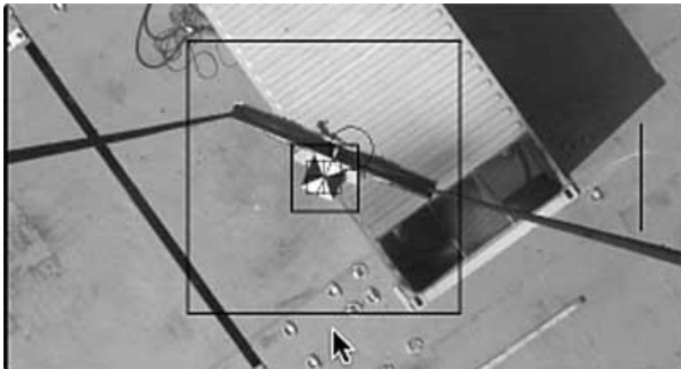
Figure 3-14 Image displayed in the cabin, which shows the position of the target and the correct vertical position as an overlaid circle (Wilson, 2012)
