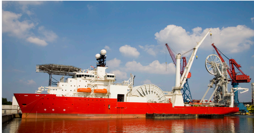
Figure 5: Cable laying vessel
