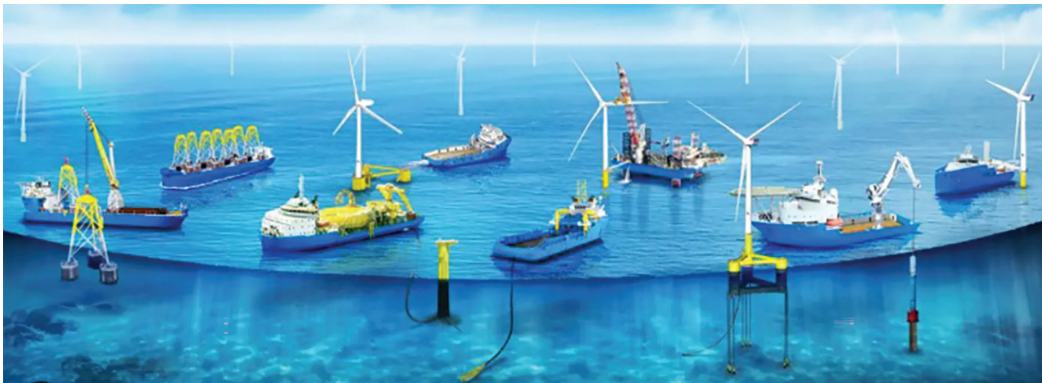
Figure 9: Illustration of various vessels and offshore wind foundation types
